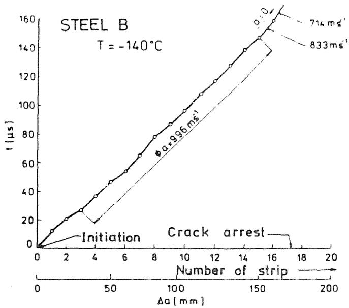
Fig. 12 - Crack length, a-time, t history, steel B.
