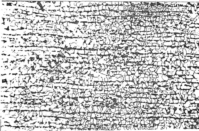
Fig. 4 - Ferrite-perlite microstructure of steel B, 500X.
