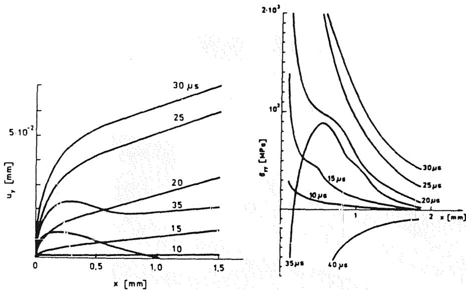
Fig. 9 - Normal stress  $\sigma_{yy}$  behaviour at the crack tip and crack profiles.
