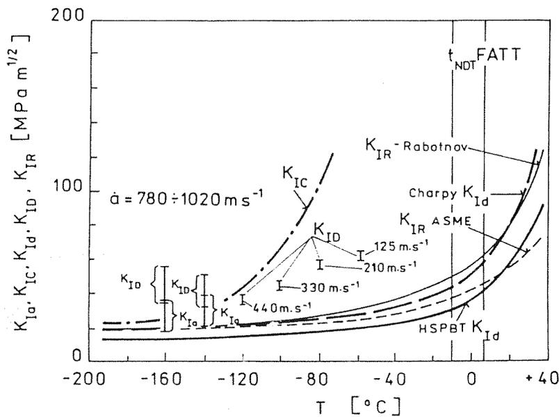
Fig. 16 - Temperature dependence of fracture toughness, steel A.
