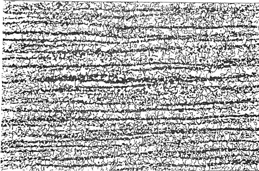
Fig. 3 - Ferrite-perlite microstructure of steel A, 500X.
