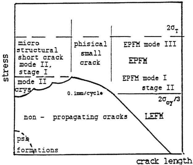
Fig. 2 The fatigue mechanisms map of Brown.
