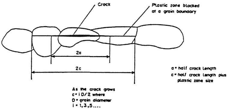
Fig.10 Schematic of a crack and blocked slip band.
