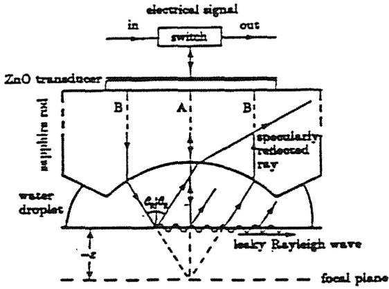
Fig.6 The acoustic lens and main acoustic waves.
