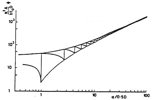
Fig.11 Oscillating pattern of the plastic displacement at the tip of a short crack.
