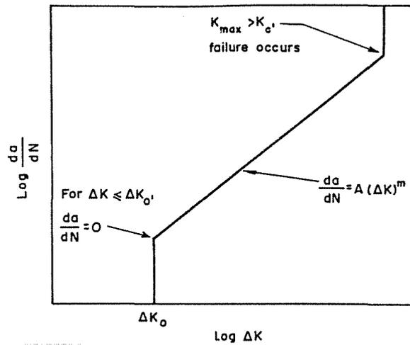
Fig.3. Assumed fatigue crack propagation relationship.
