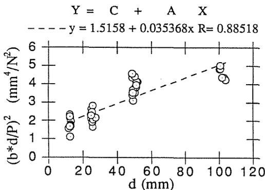
Fig. 5.b Linear regression plot for granite acc. to Bazant.
