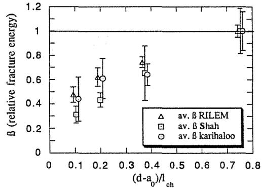
Fig. 6.a Ligament length influence on fracture energy for marble.
