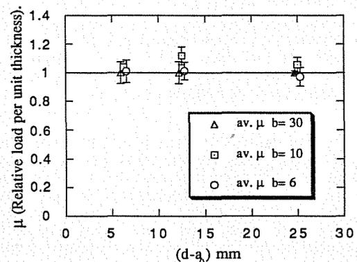
Fig. 3.b Thickness effect upon relative load for granite.
