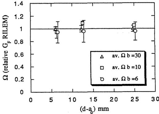
Fig. 3.d Thickness effect upon fracture energy for granite.
