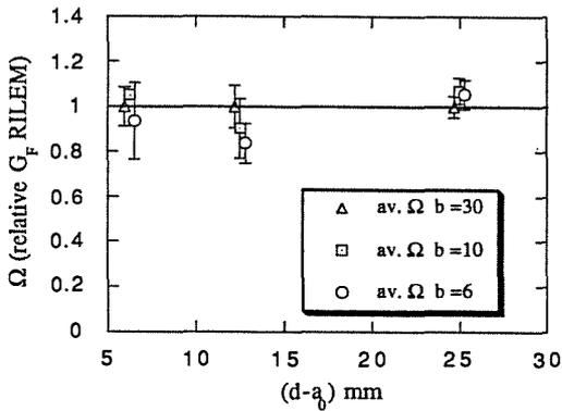
Fig. 3.c Thickness effect upon fracture energy for marble.
