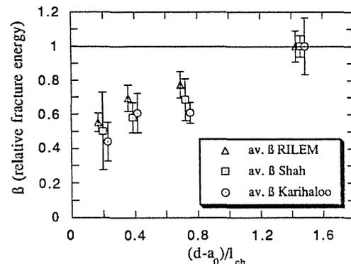
Fig. 6.b Ligament length influence on fracture energy for granite.
