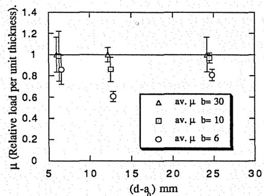
Fig. 3.a Thickness effect upon relative load for marble.
