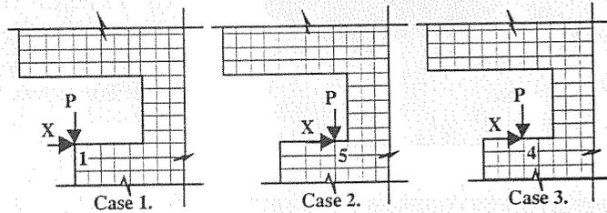
Fig. 10. Simplified loading cases. The horizontal force  $X$  is set equal to  $0.3 P$  (friction coefficient  $=0.3$ ) until the horizontal displacement fills the initial gap between steel and granite. Subsequent loading proceeds at fixed horizontal displacement of the loaded node.
