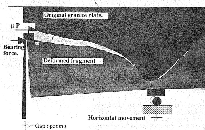
Fig. 12. Failure process in the pull-out plane stress problem: Initial cracking proceeds under frictional contact force  $\mu P$ , while the gap between the granite and the anchor decreases and the crack grows downwards (light grey picture). When the gap is exhausted, a horizontal bearing force appears that prevents further horizontal displacements, and the crack kinks upward (dark grey picture).
