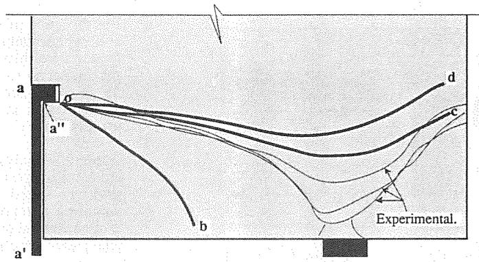
Fig. 9. Crack patterns for various boundary conditions. **ob**: crack path for no horizontal forces. **oc**: crack path for zero horizontal displacement along  $oa''$ . **od**: crack path for zero horizontal displacement along  $aa'$ .
