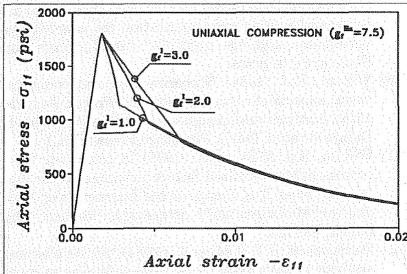
Fig. 7. Mixed-mode cracking in a uniaxial test with different values of  $g_f^I$ .
