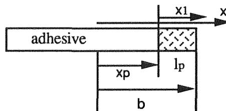
figure 3 Local reference frame with plastic zone
