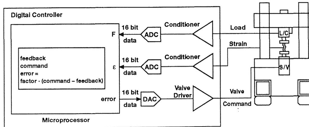
Figure 3. Calculated Variable Control
