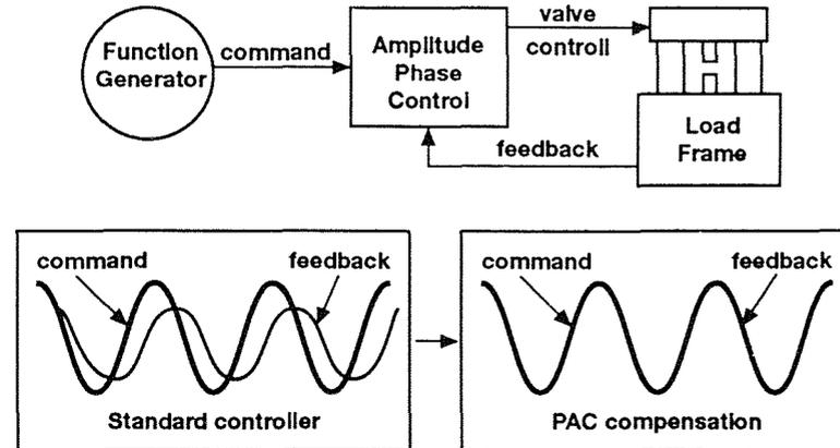
Figure 5. Phase Amplitude Controller (PAC)
