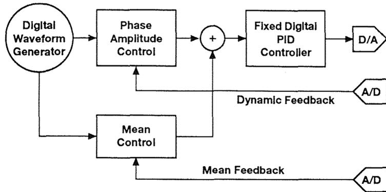
Figure 4. Phase Amplitude Controller (PAC) Mixed Mode (PAC) utilizes three separate feedbacks in a cascaded control loop. Displacement for stable control
