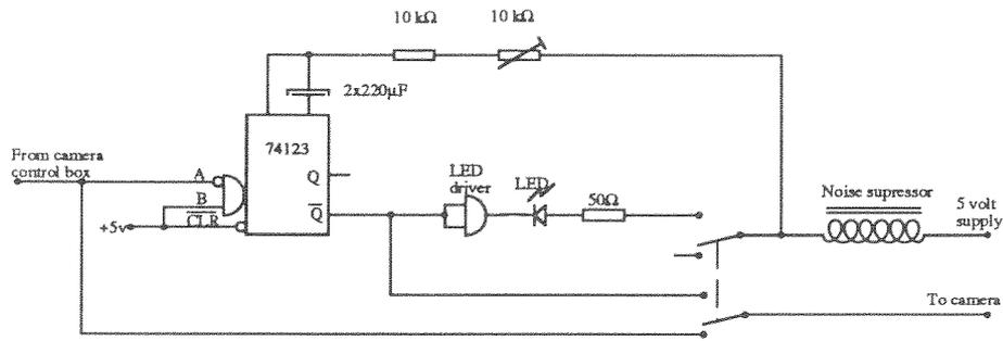
The lower change over switch directs the shutter opening signal either directly through to the camera (lower position), or through the circuit. The circuit is connected to power permanently, but the LED is disconnected when in by-pass mode. This to minimise electric noise while switching from one position to the other. Noise absorbing capacitors are not shown.
