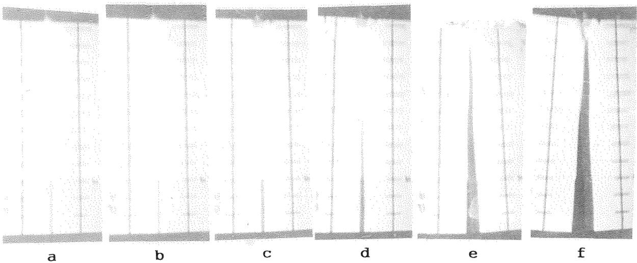
Fig. 7. Crack Propagation in Plexy Glass. The time increments between pictures is 160 micro-seconds for a-b-c-d and 400 micro-seconds for d-e-f.
