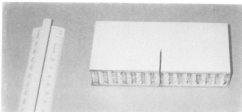
Fig. 9. Composite Specimen
