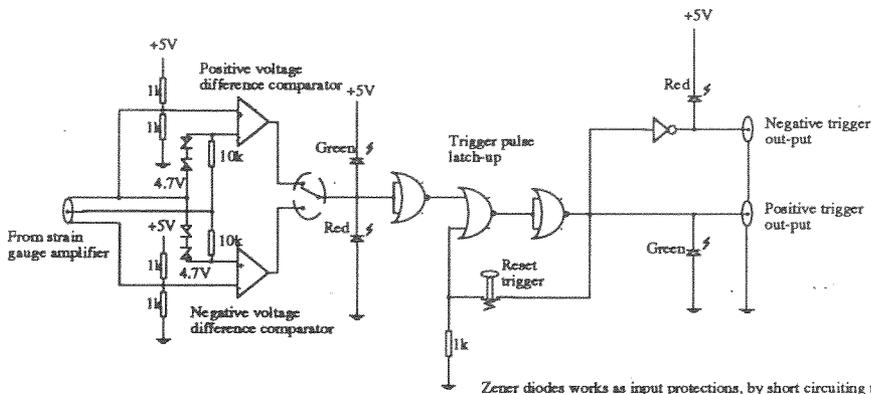
The LED's after the op-amps shows the polarity of the input signals, relative to the triggering polarity. Red LED- no trigger action and green LED - trigger action. Both LEDs on, no or very small input voltage difference.
