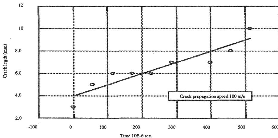
Fig. 11. Crack Growth in Composite
