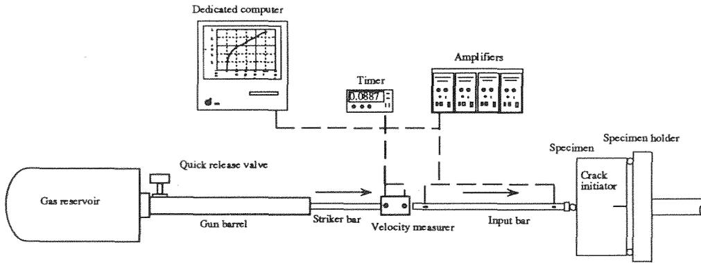
Fig. 1. Schematic View of Lateral Three Point Bending Impact Rig
