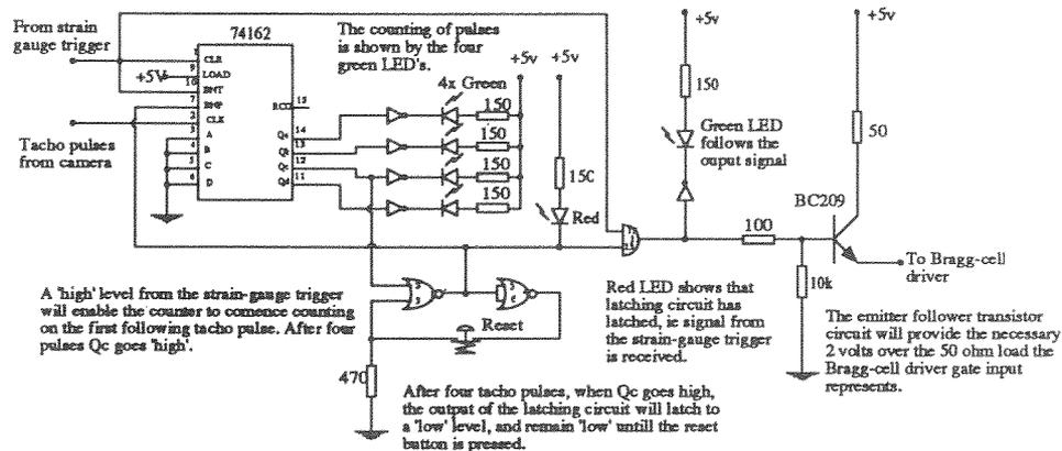
A 'high' level from the strain-gauge trigger will enable the counter to commence counting on the first following tacho pulse. After four pulses Qc goes 'high'.
