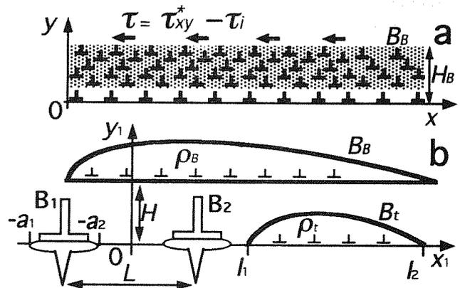
Fig. 4. The scheme (a) and the basic model (b) of a coarse shear band as a scene for development  $t$ - and  $l$ -decohesion cracking. The assemblage  $B_B$  of the upper-floor pileups of a band is shadowed in (a).
