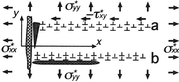
Fig. 1. Two modes of microcracking in unrelaxed coarse slip bands blocked at an impenetrable obstacle (a — *t*-cleavage, b — *l*-separation)
