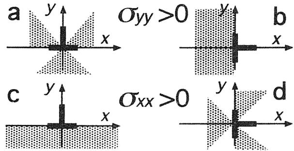
Fig. 2. Stress-fields of edge dislocations (a, b — stress  $\sigma_{yy}$ , c,d — stress  $\sigma_{xx}$ ). Areas of positive (tensile) stresses are shadowed and on borders between sectors the correspondent stresses are zero.
