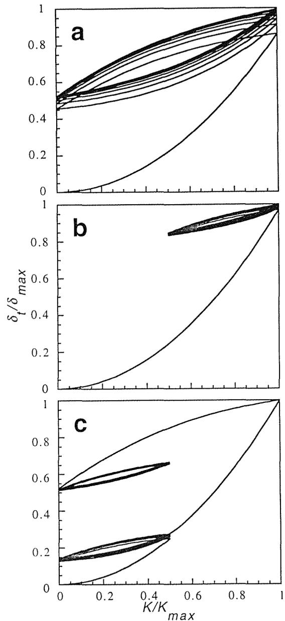
Fig. 3. Variation of CTOD vs. applied  $K$ : (a) load case I; (b) load case III; (c) load case IV.
