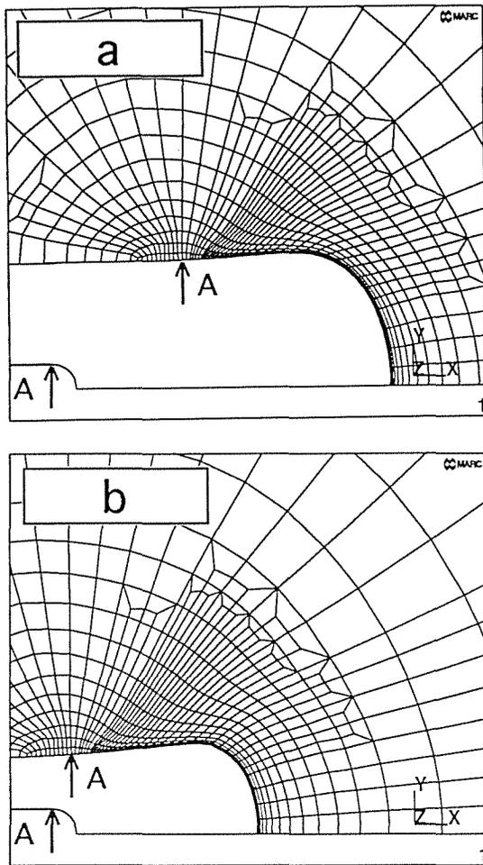
Fig. 2. Near-tip deformations at different stages of load case I: (a) at the 4th maximum load point,  $K = K_{max}$ ; (b) at subsequent unloading point,  $K = 0$  (the original crack tip is shown in the bottom left corners).
