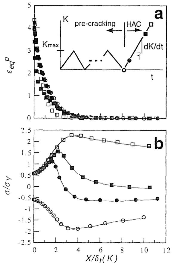
Fig. 1. Distributions of  $\epsilon_{eq}^p$  (a) and  $\sigma$  (b) along the crack line at consecutive instants of the loading history marked by corresponding symbols in the inserted scheme of the loading path.
