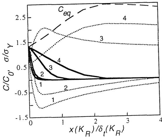
Fig. 4. Finite element solutions for concentration (solid lines) and hydrostatic stress (dotted lines) beyond the crack tip at different times under dynamic load at  $K \bullet = 1.5 \text{ MPam}^{1/2}/\text{min}$ . The dashed line shows the equilibrium concentration distribution. Curves 1-4 refer respectively to times of 180, 300, 1000 and  $t_R=2400 \text{ s}$ .
