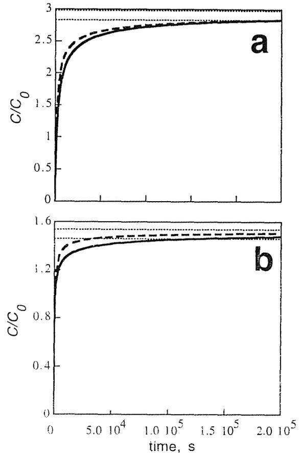
Fig. 3. Concentration evolutions according to the finite element solution (solid curves) and asymptotic one (9) (dashed curves) at sustained load: (a) in the points of maximum tensile stress  $x_{m\sigma}$ ; (b) in the high plastic strains region at  $x_{m\epsilon}$ . Horizontal lines mark the 5%-tolerance band near the corresponding equilibrium concentration levels  $C_{eq}(x)$ .
