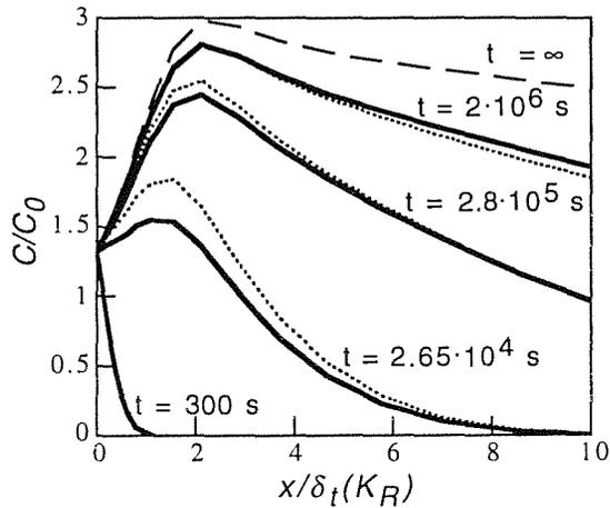
Fig. 2. Concentration distributions along the crack line under sustained load conditions: finite element solution (solid lines) and asymptotic one  $C_{al}(x)$  (dotted lines). The dashed line shows the  $C_{eq}$ -profile.
