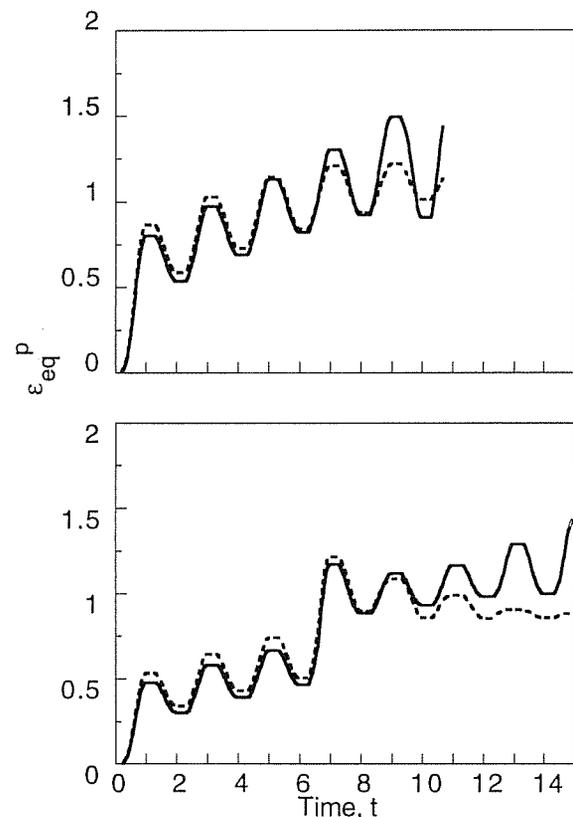
**Fig. 8.** Typical variations of the equivalent plastic strain near the crack tip in the material points at about the same distance from the tip contour during constant amplitude cycling (load case II, top graph) and in fatigue with an overload peak at  $t = 7$  (load case III, bottom figure) in the shear band (solid lines) and in the wedge-shaped zone between the bands (dashed curves).
