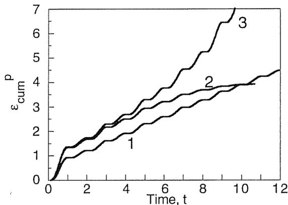
**Fig. 6.** Typical patterns of the cumulative plastic strain near the crack tip under constant amplitude cycling in the material points at about the same distance from the tip contour: (1) at the tip apex when shear bands do not arise, load case I; (2) and (3) respectively, in the shear band and at the tip apex belonging to the wedge-shaped zone between the bands, load case II.
