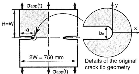
Fig. 1. The model testpiece geometry and applied load.
