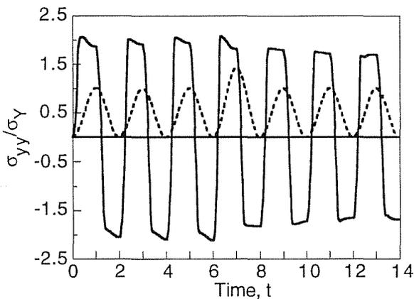
Fig. 4. Evolution of the axial stress ahead of the crack tip under sine-shape pattern of the applied loading route III with an overload peak at  $t = 7$  ( $N = 4$ ) shown by the dashed line in arbitrary units A combined isotropic-kinematic rule for strain-hardening was used in this case.
