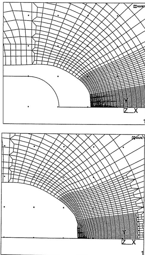
**Fig. 2.** Crack tip deformations at the third cycle of the loading route II with kinematic strain-hardening: (top) at the beginning of the cycle with  $K = 0$ ; (bottom) at  $K = 0.8K_{max}$  during subsequent forward load course. The grid spacing is  $2.5 \mu\text{m}$  in both; the undeformed crack tip is shown in the bottom-left corner of the former one.
