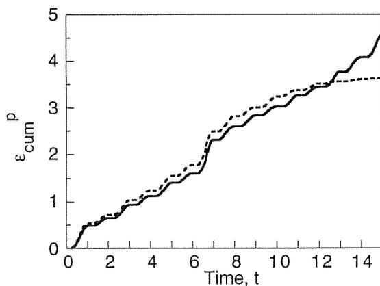
**Fig. 7.** Cumulative strain evolutions in the material points at about the same distance from the tip contour during fatigue with an overload peak at  $t = 7$  (load case III) in the shear band (solid line) and in the wedge-shaped zone between the bands (dashed curve).
