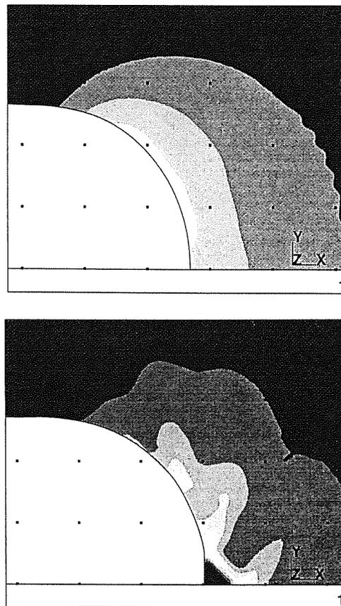
**Fig. 3.** Distribution of equivalent plastic strain rate near deformed crack tip when  $K_{max}$  is attained during the initial monotonic load stage of the loading regime II: (top) isotropic hardening; (bottom) kinematic hardening. Identical equidistant-section bands with  $\xi_{eq}^p$  increase from dark to bright in arbitrary units; the grid spacing is  $2.5 \mu\text{m}$  in both pictures.
