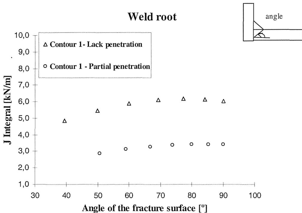
Fig. 4 – Variations of the J integral at the weld root against the angle of the fracture plane (angle of the fatigue crack).
