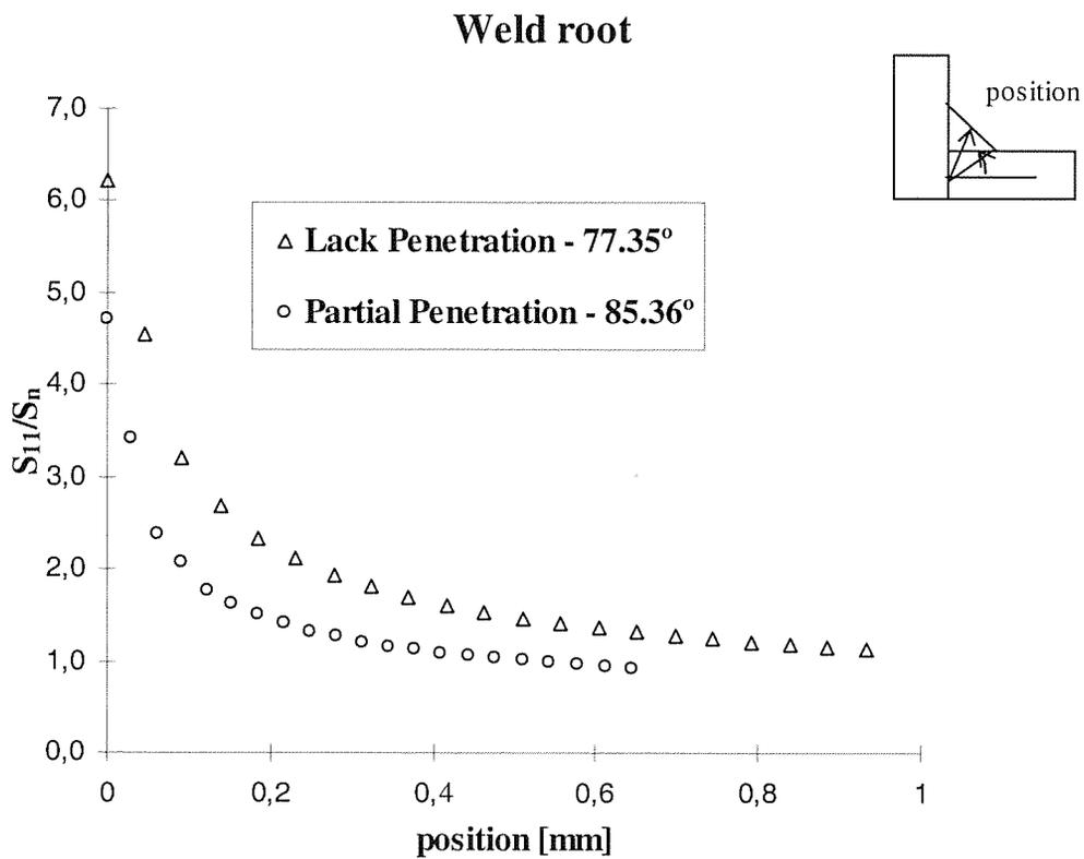
Fig. 3 – Variation of the stress concentration factor,  $K_t$ , against the polar distance,  $r$ , measured from the welded root in the directions of maximum stress.  $S_{11}$  – maximum normal stress in the loading direction, 1.  $S_n$  – nominal stress in the loading direction, 1.
