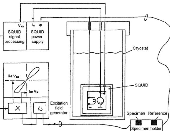
Figure 1. Eddy current measuring device with SQUID
