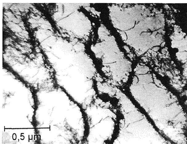
Figure 7. Dislocation cell structure after 3205 cycles, specimen Nb-I-3
