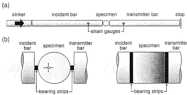
Figure 3: Experimental set-up (a), and detail of the specimen (b).
