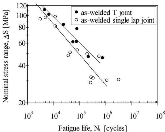
**Fig. 3.** As-welded joints' experimental fatigue results.
