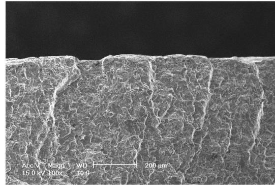
**Fig. 8.** Multiple initiation in single lap joints.
