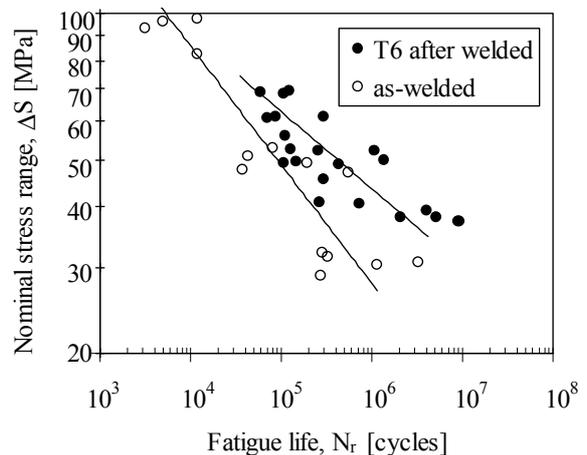
**Fig. 5.** Single lap joints' experimental fatigue results.
