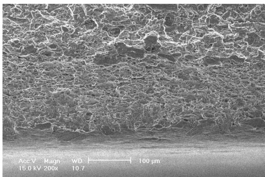
**Fig. 7.** SEM micrograph of the heat-treated joint's rupture zone.
