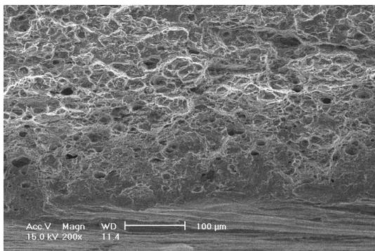
**Fig. 6.** SEM micrograph of the as-welded joint's rupture zone.
