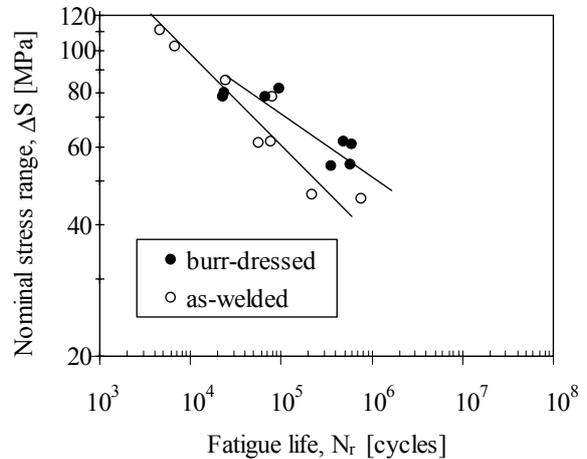
**Fig. 4.** T joints' experimental fatigue results.
