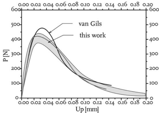
**Fig 10** – Force –displacement plot of a SENB sample with notch length  $a = 5$  mm.
