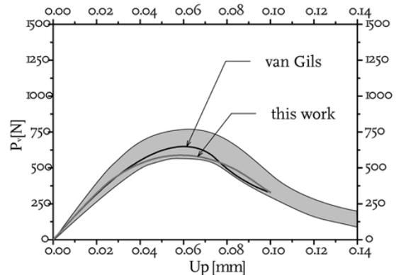
**Fig 9**– Force –displacement plot of a WOL sample with notch length a = 90mm.
