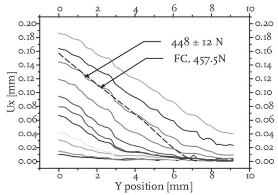
**Fig. 7** – Experimental data and fictitious crack fitting of the crack profile of samples in water at 45 °C
