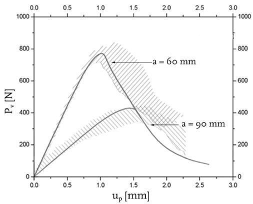
**Fig. 5** – Experimental data and fictitious crack fitting of WOL samples in water at 45 °C with two different notch lengths
