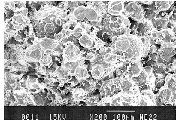
**Fig 2.** - Microphotograph of the NZS material, where it is seen the PMMA beads bonded together.
