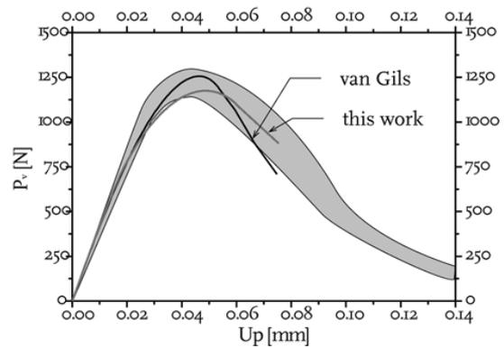
**Fig 8** –Force –displacement plot of a WOL sample with notch length a = 60mm.
