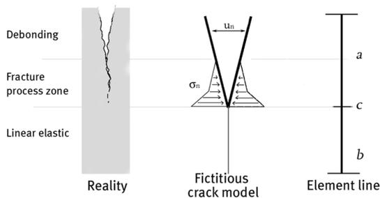
**Fig 1.** - Sketch of the fictitious crack concept. At the left is the real crack, in the middle is the fictitious crack modelling, and at the right is the element line with its three different labelled regions. In the computation, three regions are differentiated: before the crack tip (b), the crack tip (c) and after the crack tip (a)
