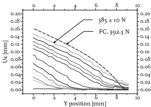
**Fig. 6** – Experimental data and fictitious crack fitting of the crack profile of dry samples at room temperature
