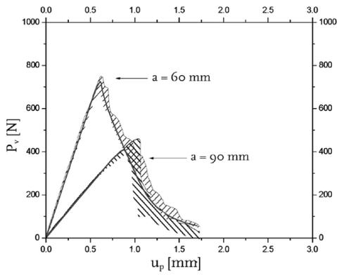
**Fig. 4** –Experimental data and fictitious crack fitting of WOL samples at room conditions with two different notch lengths
