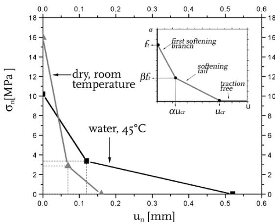
**Fig 3.-** Softening curves of the FC simulation for the two conditions of the PMMA-based materials
