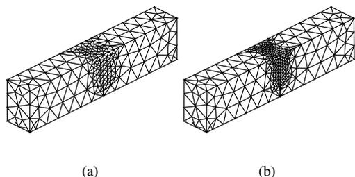
Figure 2: The meshes used in the simulations for specimen A1 ( $D = 75$  mm); element size at middle surface (a) 6 mm; (b) 3 mm.
