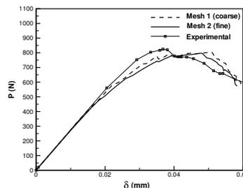
Figure 3: The load curve comparison for mesh 1 and 2 and compared with experimental results.
