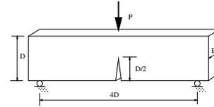
Figure 1: A concrete beam subjected to three point bending.
