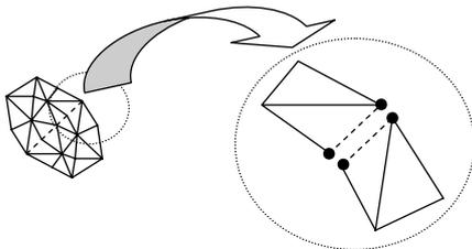
**Fig. 1.** Zero-thickness interface element with double nodes inserted into the Continuum FE mesh.
