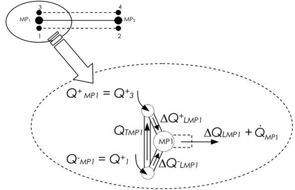
Fig. 4. Distribution of leak-off flow rate between longitudinal and transversal mid-plane flow rates.
