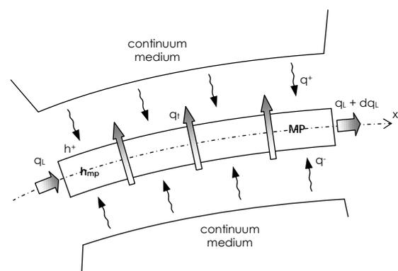
**Fig. 2.** Flow through the differential joint element.
