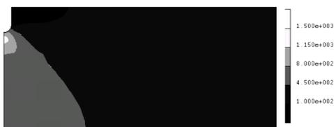
**Fig. 3.** Hydrostatic stress distribution in a bar under traction indicating homogenization of the stress-state away from the notch and obtained with the finite element code MSC.MARC.
