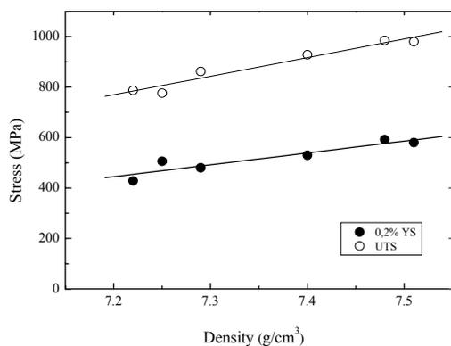
Figure 3. Effect of density on tensile properties.
