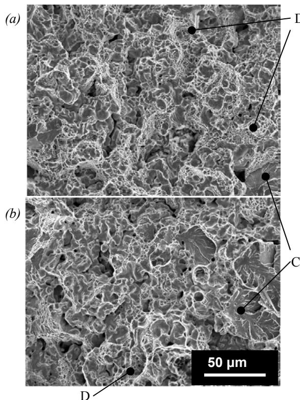
Figure 4. SEM micrograph showing dimples (D) and cleavage (C) on the fracture morphology of (a) material 1 ( $\rho = 7.22$  g/cm³) and (b) material 4 ( $\rho = 7.51$  g/cm³).
