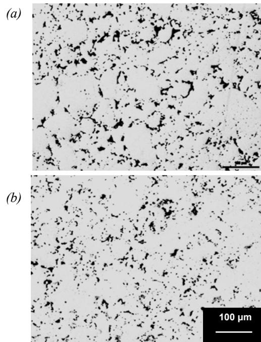
Figure 1. Typical porosity in (a) material 5,  $\rho = 7.29$  g/cm<sup>3</sup>; (b) material 6,  $\rho = 7.51$  g/cm<sup>3</sup>.
