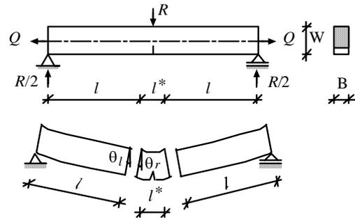
Figure 2. Cracked Beam-column under Tension.
