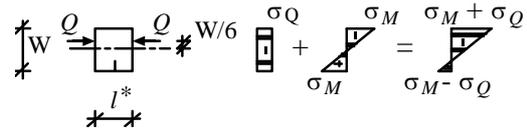
Figure 4. Normal Stress over Uncracked Section .
