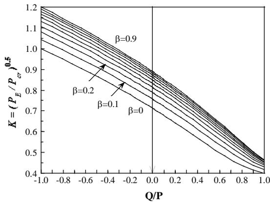
Figure 6. Effective Length Factor for Weakened X-Bracing.
