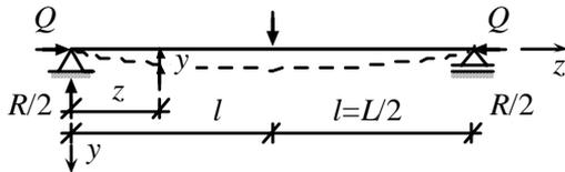
Figure 3. Cracked Beam-column under Compression.
