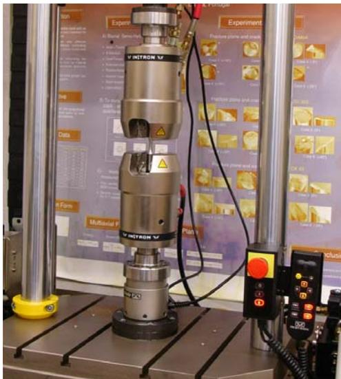
Figure 2. Biaxial testing machine (Instron 8874)
