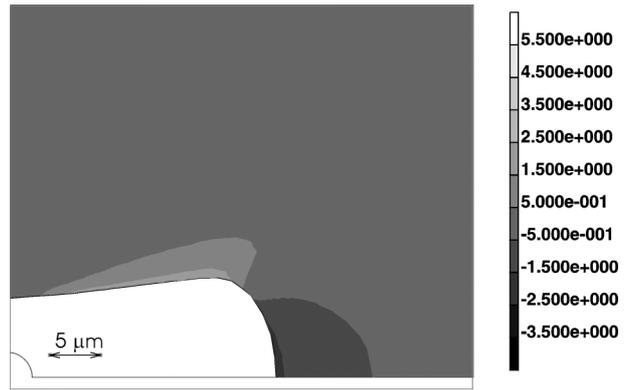
Fig. 3. Distribution of plastic strain  $\epsilon_{xx}^p$  at the end of the sixth cycle of the route II in deformed solid configuration (original tip is in the bottom-left corner).
