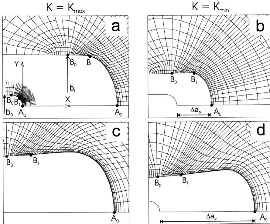
**Fig. 1.** Crack tip deformations in the double-edge-cracked panel at  $K_{max}$  and  $K_{min}$  (unloading) of the first (a,b) and the fifth (c,d) cycle of the loading route II. Undeformed tip contour is seen in the bottom-left corners in (a,b,d), and the undeformed mesh fragment is shown in (a).
