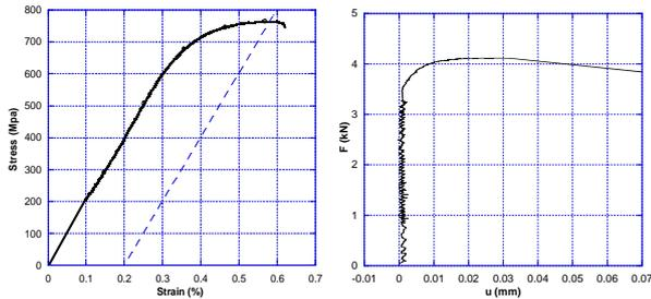
Fig. 1 Stress-strain curve and pull-out test results for wires.
