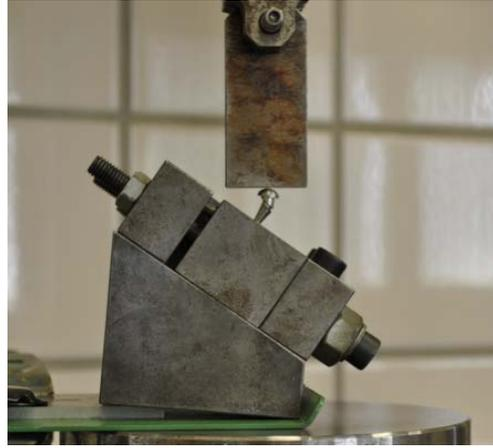
Figure 6 Hemispheric loading member configurations for pre-angled abutment test.
