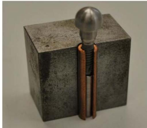
Figure 7 Clamping system with copper tube.
