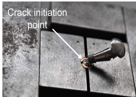
Figure 8 Failure Point.
