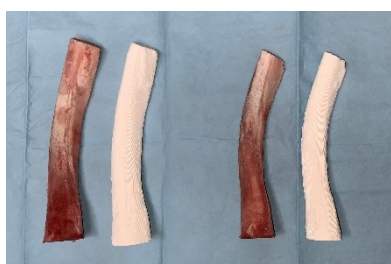
Figure 1. Porcine rib specimens and PLA simulants made through FDM.
