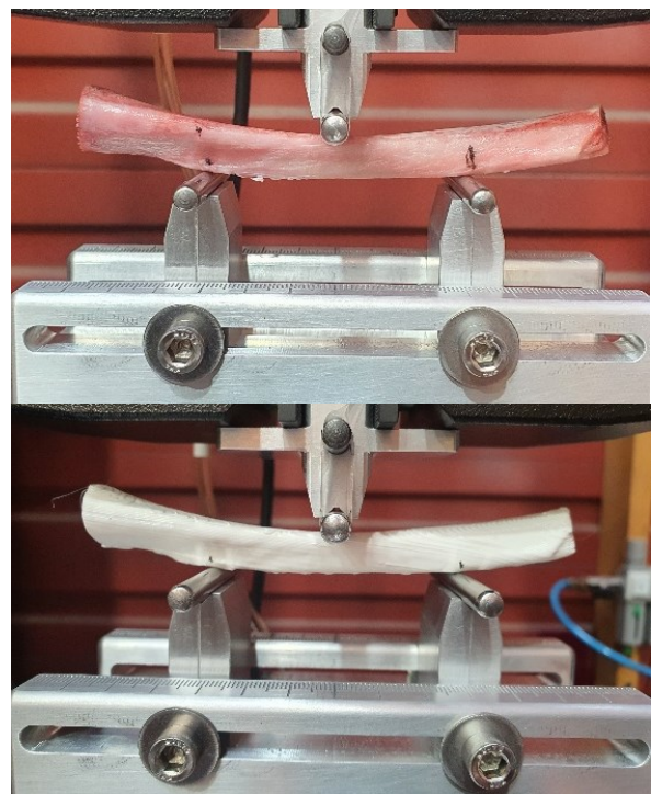
Figure 6. Three-point bending test of a porcine rib and PLA simulant.
