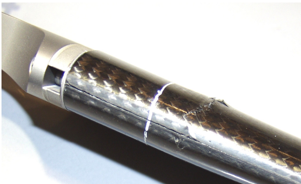
Figure 8. Compression failure of front push rod
