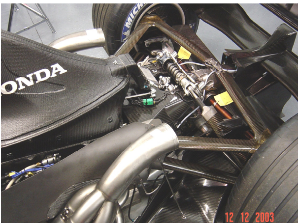
Figure 3. Composite gearbox and rear suspension
