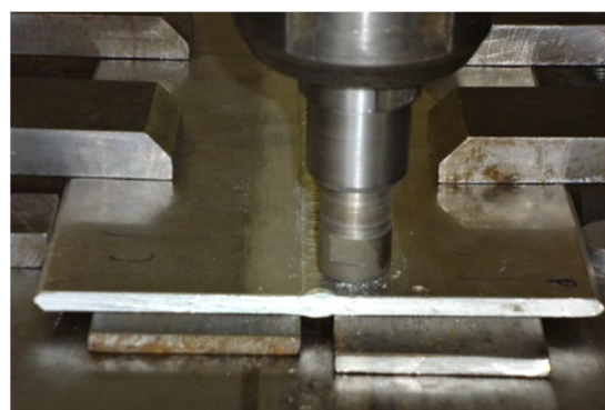
Figure 2. MIG welded plate post-processed by FSP.
