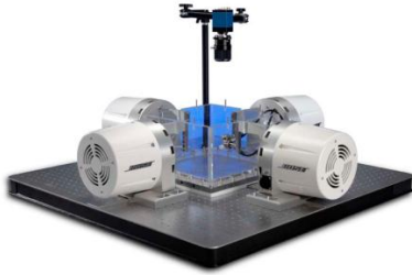
Figure 3. Biaxial testing machine from Bose with linear electrical motors, [8].
