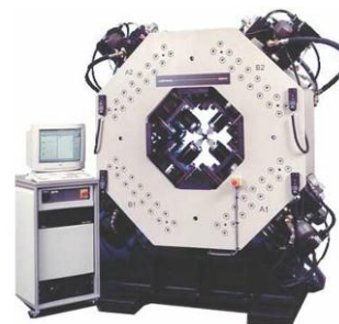
Figure 2. Biaxial testing system with four hydraulic actuators from INSTRON, [3].
