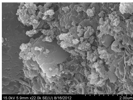
Figure 10: Aggregation of nanoCaCO 3 in 30% fly ash-cement pastes with 5% nanoCaCO 3 addition.
