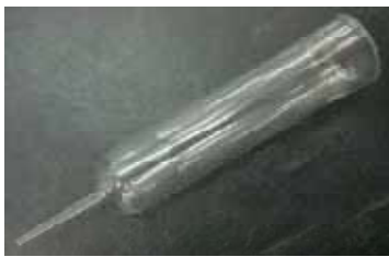
Figure 1: Image of the injection molded Pressure Vessel, including cold runner.
