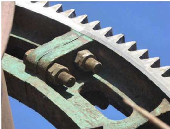
Figure 3 – Toothed crown (girth gear), composed of two halves; detail showing one of two connections.
