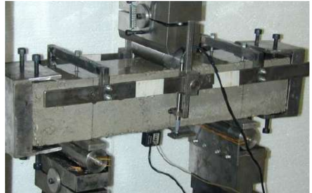
Figure 8. Three point bending test in a concrete sample.
