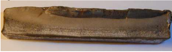
Figure 9. Fractured section of TDR8 Specimen.
