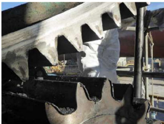
Figure 4 - Toothed crown and pinion. The teeth of the pinion show plastic flow of material outside the teeth width; at a lower scale this also existed in the toothed crown but that plastically deformed material was removed during the present stoppage.
