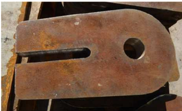
Figure 9 – New eyebars designed by Leca / Avelar
