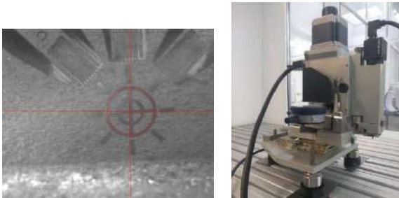
Figure 2. Strain gague rosette centering and Hole-Drilling equipment.
