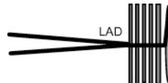
Fig. 8. Micromechanism of LAD by anodic dissolution of the fibers or plates (mode I crack growth) and posterior mechanical fracture of a slender pearlitic pseudocolony.
