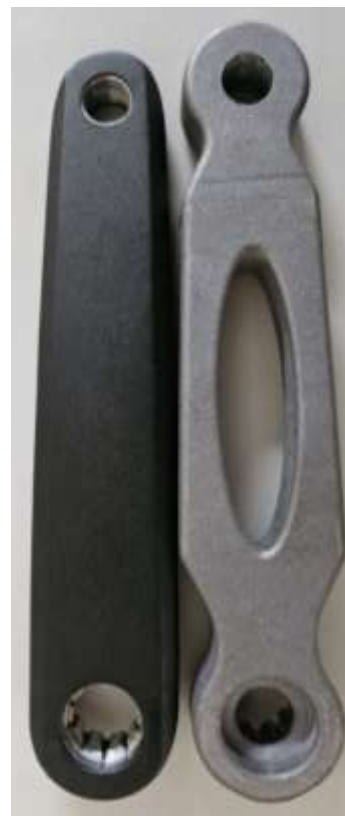
Figure 3. Comparison between cranksets produced by L-PBF and the Miranda® brand.
